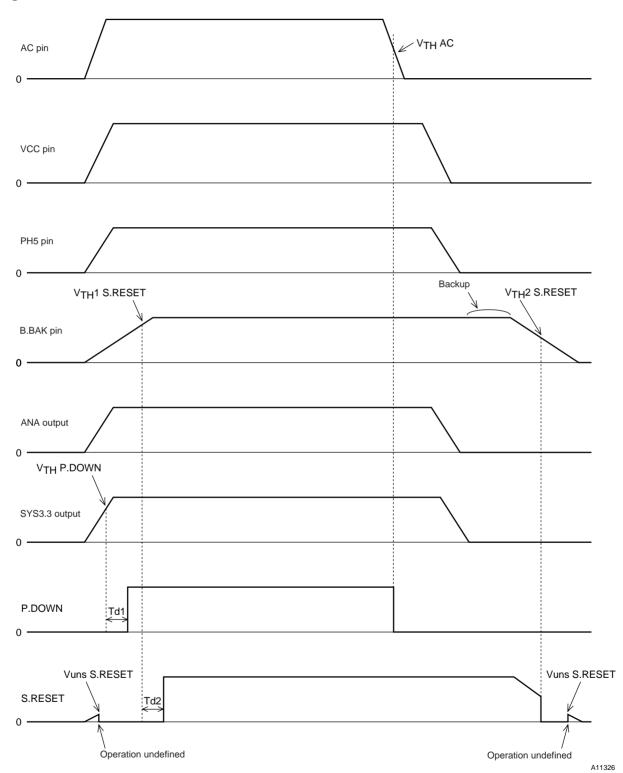
$\label{eq:Note:the S.RESET output has an undefined operating state, so care is required in application design.$
