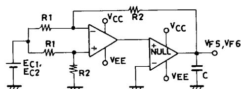
$$CMR = 20 \log \left| \frac{(E_{C1} - E_{C2})(1 + R_2/R_1)}{V_{F5} - V_{F6}} \right|$$
