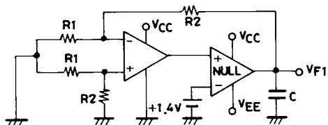
$$V_{IO} = \frac{V_{F1}}{1 + R_2/R_1}$$
