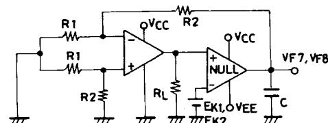
$$VG = \frac{(E_{K1} - E_{K2})(1 + R_2/R_1)}{V_{F8} - V_{F7}}$$
