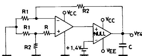
$$I_B = \frac{V_{F4} - V_{F3}}{2R (1 + R_2/R_1)}$$
