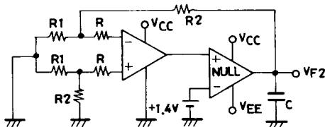
$$I_{IO} = \frac{V_{F2} - V_{F1}}{R (1 + R_2/R_1)}$$
