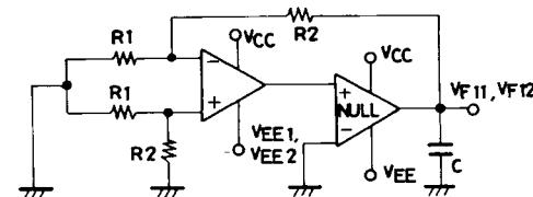
$$SVR (-) = 20 \log \left| \frac{(1 + R_2/R_1)(V_{EE1} - V_{EE2})}{V_{F11} - V_{F12}} \right|$$
