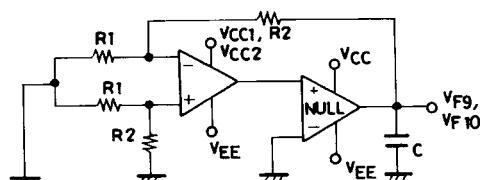
$$SVR (+) = 20 \log \left| \frac{(1 + R_2/R_1)(V_{CC1} - V_{CC2})}{V_{F9} - V_{F10}} \right|$$
