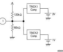
GND < pin 1 level - DC < 1.0 V: TRICK2 1.0 V < pin 1 level - DC < 3.0 V: NORMAL 2.0 V < pin 1 level - DC < 5.0 V: TRICK1
