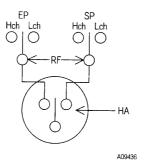
Comparator Output: Pin 2 EP envelope > SP envelope: High (min. 4.0 V) EP envelope < SP envelope: Low (max. 0.7 V)
