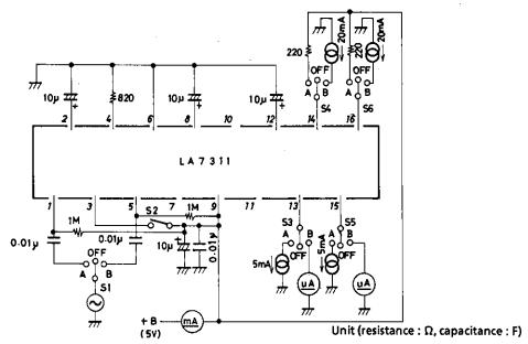
Note: Remove the  $1M\Omega$  resistor connected across pins (1) and (9) and across pins (5) and (9) except when measuring  $\Delta V_P$ ,  $\Delta V_R$ ,  $V_{12}$ ,  $V_{1N}$ .
