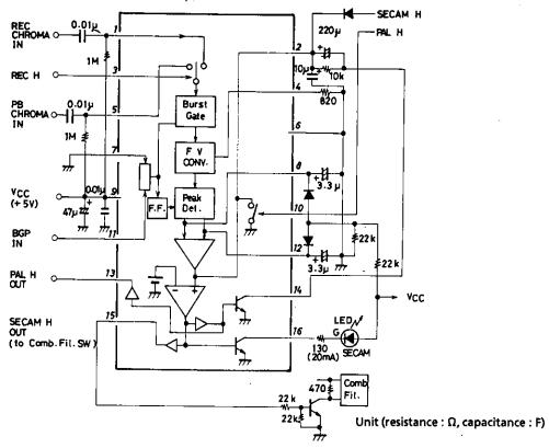
Note 1: When the BGP is positive, apply an input to pin 7 and connect pin 11 to  $V_{CC}$ . Note 2: When pin 10 is not in use, bring pin 10 to the open state or connect to GND.
