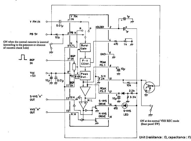
Adjustment method: Adjust the VR (from VR center position) connected to pin 4 so that the DC voltage on pin 8 becomes 2.0V when the FM-Y signal at the (normal) VHS REC tape PB mode is input.
