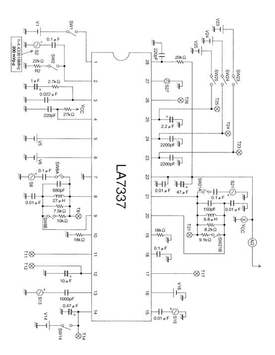
Note: Use an FET probe when measuring T8, T21, and BGP.
