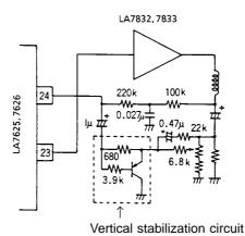
Unit (resistance:  $\Omega$ , capacitance: F)
