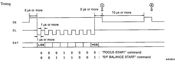
When sending a TRACK-OFFSET ADJUST START command or a FOCUS-OFFSET ADJUST START command after either  $V_{CC}$  ON (POWER ON RESET), RESET command, or a corresponding OFFSET ADJUST OFF command, waiting time is necessary as listed below. (Only when a 4.2 MHz clock is input.)
