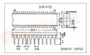
Level Meter Driver for 12 LEDs
