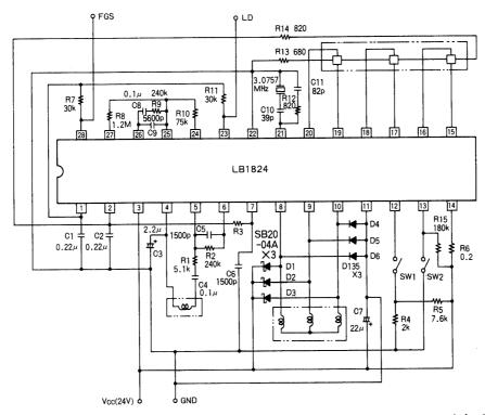
Unit (resistance:  $\Omega$ , capacitance: F)
