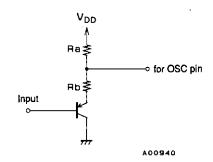
Use the LB1870  $V_{REG}$  output for the  $V_{DD} = 6.3 \text{ V}$  case.
