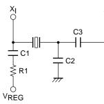
C1, R1 : For stable oscillation C2 : For overtone oscillation prevention C3 : For crystal coupling
