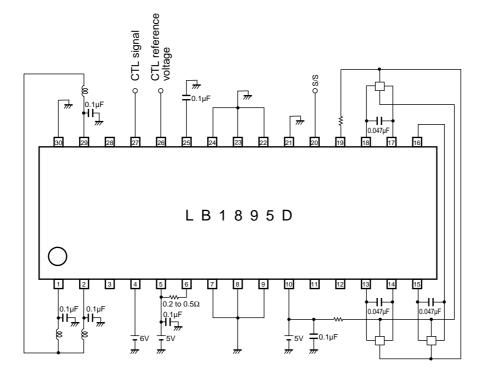
Between power supply and GND, Output and GND, and between Hall inputs: The capacitors may change, depending on the motor. The capacitor between the Hall inputs in particular may not be required with some motors. A06728
