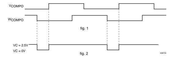
If braking is applied according to the value obtained by OR logic in  $V_{COMPO}$  and  $W_{COMPO}$  together, for example, reverse braking is applied according to the following timing.
