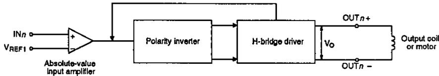
The reference voltage,  $V_{REF1}$ , from the CD player's DSP, is boosted to 3.9 V ( $1/2 V_{CD2}$ ). The actuator's voltage characteristic is shown in the following figure.
