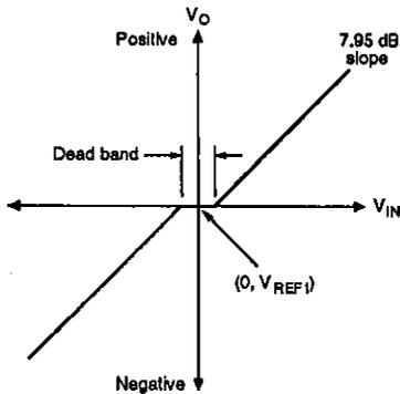
The V-type actuator driver, using  $V_{REF1}$  as a reference, generates a reverse polarity output. Note that there is a dead band in the range  $V_1 = V_{REF1} \pm 100$  mV (max) where  $V_O$  remains constant. The driver also incorporates a feedback loop for accurate gain.
