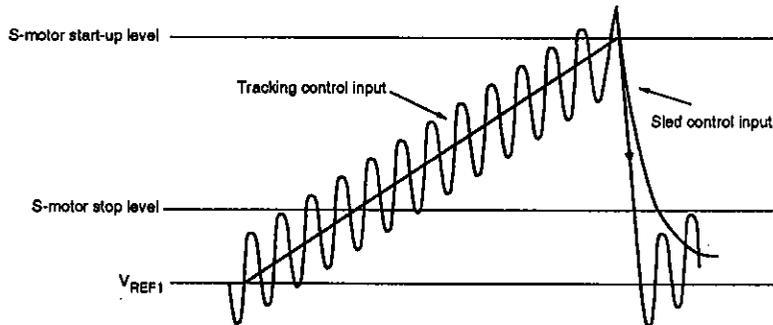
The voltage characteristic of the sled actuator driver in step mode is shown in the following figure. In step mode, maximum voltage is applied to the H-bridge. Note that the control input is usually lower than  $V_{REF1}$ .
