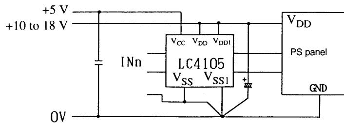
Keep the impedance of the  $V_{SS}$  and  $V_{SS1}$  lines as low as possible. Connect a large electrolytic capacitor across the  $V_{DD1}$  and  $V_{SS1}$  pins and close to the IC. Wherever possible, keep the grounds for the power supply circuits and the signal circuits separate and connect the two at a single point.
