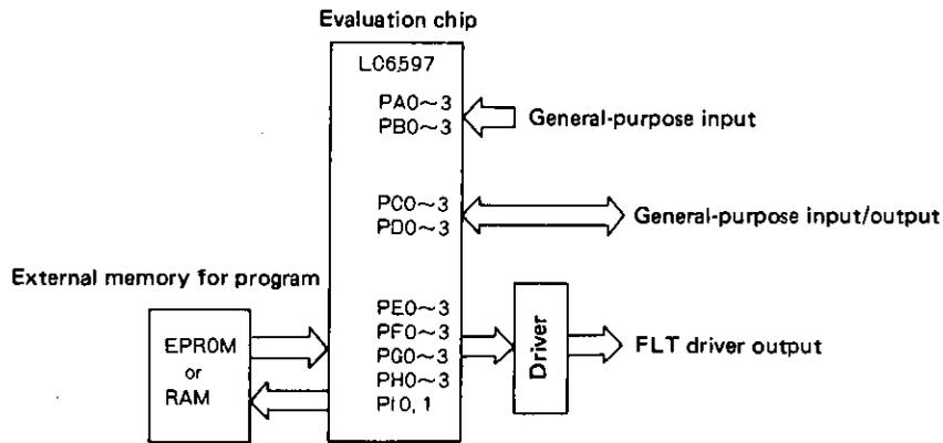
Fig. 1-1 Basic evaluation system using evaluation chip
