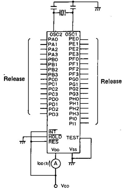
Fig. 4 I<sub>DD(3)</sub> test circuit
