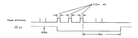
When the phase difference between the programmable and reference divider outputs exceeds 3.2 $\mu$ s. The  $\overline{UL}$  line is held low for 6ms after the last out-of-range phase sample is detected, as shown below.
