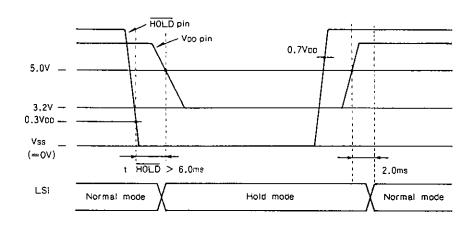
VDD must remain at 5.0V or higher (crystal oscillator requirement) for 6.0msec (tHOLD) after the HOLD line is asserted (HOLD<0.3VDD). After this VDD may go as low as 3.2V. There are no constraints on timing when the chip is leaving hold mode.
