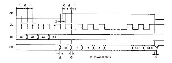
3) In mode 3: The serial data output mode (mode 3) is selected by specifying the mode select data (4 bits). Setting CE high allows I₀ to be output to DO. Once CE is put high data is output to the DO pin when the internal shift register contents shift
