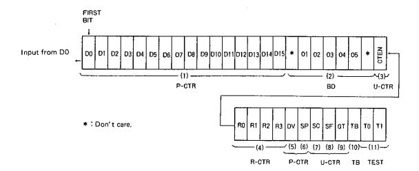
The control serial data of LC7216M consists of 36 bits. When power is turned on, data should be entered on every one of these bits for initialization. However, the last two bits are not related to the user, because data on these bits is used for switching the test mode.
