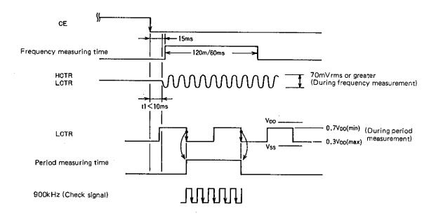
The DO pin is forcibly set high when the universal counter starts counting (CTEN=1), and automatically goes low after the measurement is finished (i.e., after 120 or 60msec, or a signal input in 1- or 2-cycle). DO can, therefore, be used to check the measured value.
