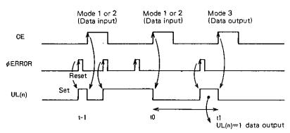
Internal data UL(n) is set/reset on the positive transition of  $\phi$  ERROR signal/CE signal, respectively. In mode 3 (data output),  $\phi$  ERROR data UL(n) after the previous positive transition of CE signal is read. In the example shown above, data for the period of  $t_0$  to  $t_1$  is read.
