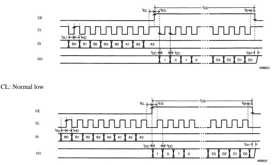
Notes:1. Since the DO pin is an n-channel open-drain output, the transition times (t<sub>DC</sub>, t<sub>DH</sub>) will differ with the value of the pull-up resistor used.
