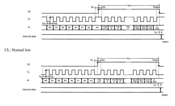
Serial data output (OUT)  $t_{SU}$ ,  $t_{HD}$ ,  $t_{EL}$ ,  $t_{ES}$ ,  $t_{EH} \ge 0.75 \ \mu s$   $t_{DC}$ ,  $t_{DH} < 0.46 \ \mu s$   $t_{CE} < 20 \ ms$  CL: Normal high
