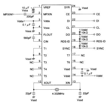
Notes: 1. Determine the value of the DO pin pull-up resistor based on the required serial data transfer speed. 2. If the SYR pin is unused, it must be connected to ground.
