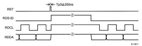
Caution: After an RST input, the RDCL and RDDA outputs stop at the high level until the first RDS ID detection.
