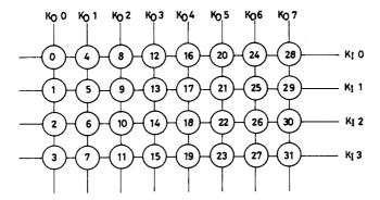
Multi-press of key No. 20 and one of key No. 21, 22, 23 may be done, with no priority given in key entry. When the two keys are kept pressed, a series of pulses will be output according to each key entry. If multi-press of keys which are not allowed multi-press is done, no output will be delivered.
