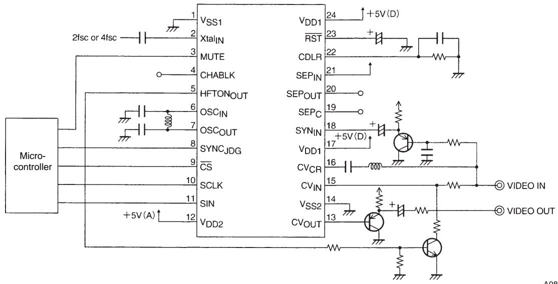
Note: When a sync tip level of 1.3 V DC (CV<sub>IN</sub> input signal: sync tip = 1.3 V) is selected for the internal generated video signals by option settings, the electrolytic capacitor connected to SYN<sub>IN</sub> must be connected with the correct polarity.
