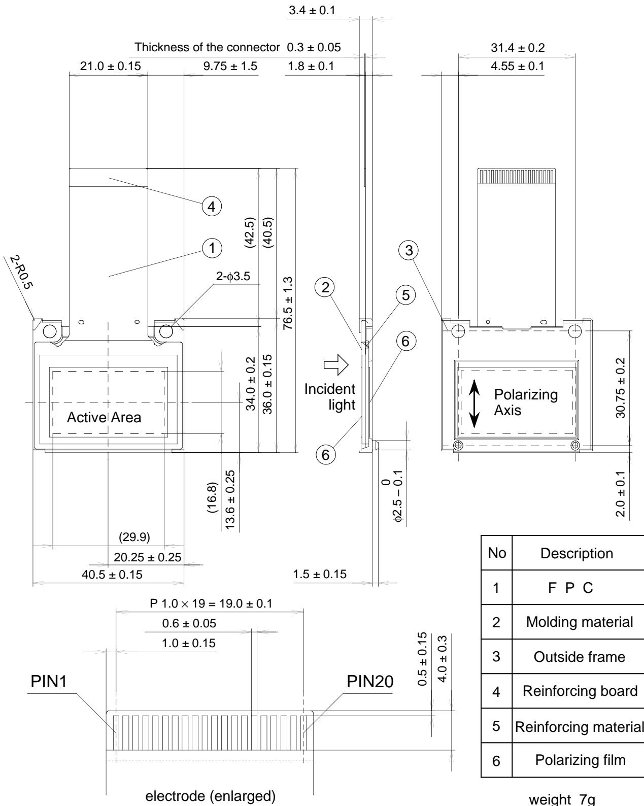
The rotation angle of the active area relative to H and V is  $\pm 1^\circ$ .
