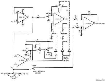
$\bullet \quad \mathsf{V}_{\mathsf{OUT}} \text{ starts from zero and is equal to the integral of the input voltage with respect to the threshold voltage:} \\$
