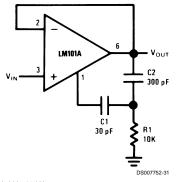
Power Bandwidth: 15 kHz Slew Rate: 1V/µs
