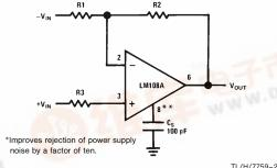
\*\*Bandwidth and slew rate are proportional to 1/C<sub>s</sub>.
