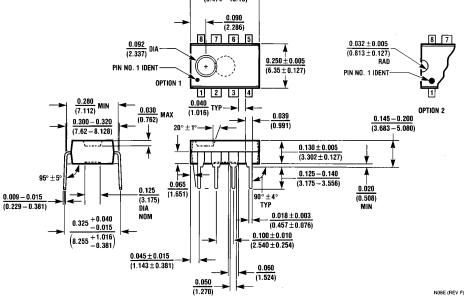
Molded Dual-In-Line Package (N) Order Number LM308AN NS Package Number N08E
