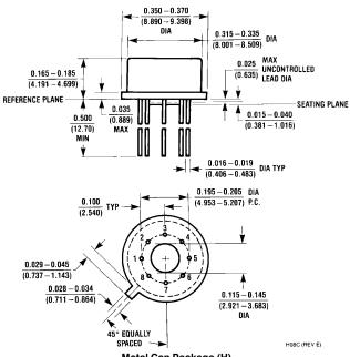
Metal Can Package (H) Order Number LM108AH, LM208AH or LM308AH NS Package Number H08C
