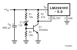
FIGURE 8. Undervoltage Lockout for Buck Regulator
