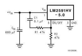
FIGURE 7. Delayed Startup
