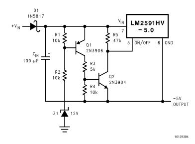
This circuit has an ON/OFF threshold of approximately 13V.
