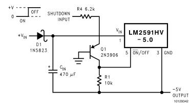
FIGURE 12. Inverting Regulator Ground Referenced Shutdown
