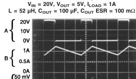
A: Output Pin Voltage, 10V/div. B: Inductor Current 0.5A/div. C: Output Ripple Voltage, 50 mV/div. Horizontal Time Base: 2 μs/div.
