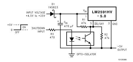
FIGURE 13. Inverting Regulator Ground Referenced Shutdown using Opto Device
