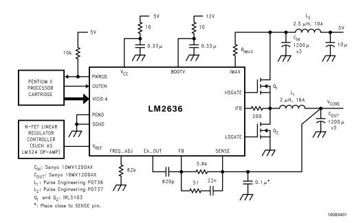
FIGURE 1. 5V to 1.3V-3.5V, 14A Power Supply
