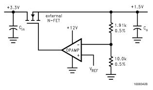
FIGURE 9. V<sub>RFF</sub> Used in an N-FET LDO Supply
