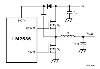
FIGURE 3. BOOTV Voltage Supplied by a Charge Pump
