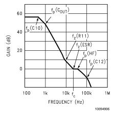
FIGURE 5. Typical Loop Gain Plot
