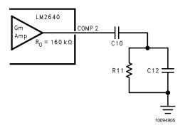
FIGURE 4. Typical Compensation Network
