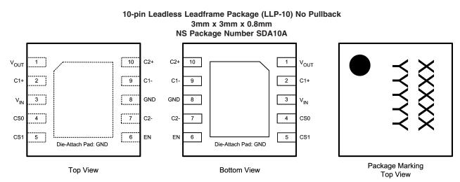
**Note**: The actual physical placement of the package marking will vary from part to part. The package marking placeholder "XXXXX" is a code for die traceability. "YYYYY" identifies the device (part number, voltage option, etc.). See the Order Information table below for the device ID codes.
