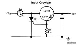
5. **Preventing latchoff** for loads connected to negative voltage:
