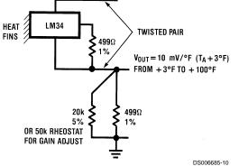
$V_{OUT} = 10 \text{mV}^{\circ}\text{F} (T_A+3^{\circ}\text{F})$ FROM +3°F TO + 100°F
