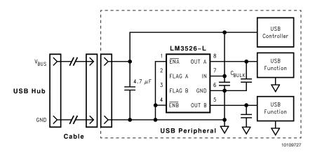
FIGURE 5. In-rush Current-limit Application
