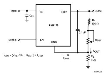
FIGURE 5. Programmable Current Source
