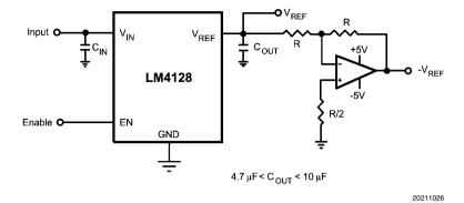
FIGURE 3. Voltage Reference with Complimentary Output
