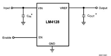
\*Note: The capacitor  $C_{IN}$  is required and the capacitor  $C_{OUT}$  is optional.
