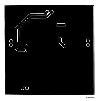
FIGURE 4. Recommended MH PCB Layout Bottom Layer
