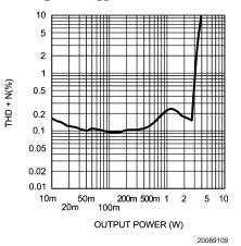
THD+N vs Output Power R<sub>L</sub> = 8 $\Omega$ , V<sub>DD</sub> = 14V, f = 1kHz
