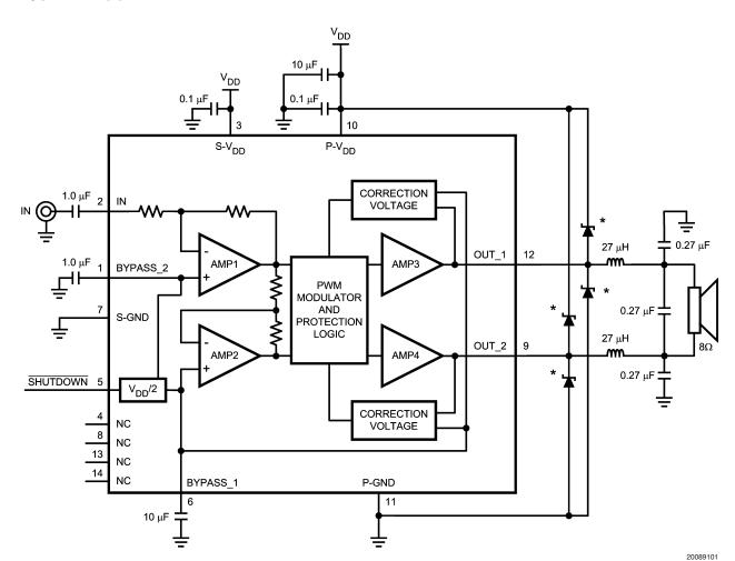
FIGURE 1. Typical Audio Amplifier Application Circuit (\* Zetex ZHCS506)
