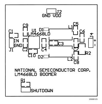
FIGURE 5. Recommended LD PCB Layout Top Silkscreen Layer
