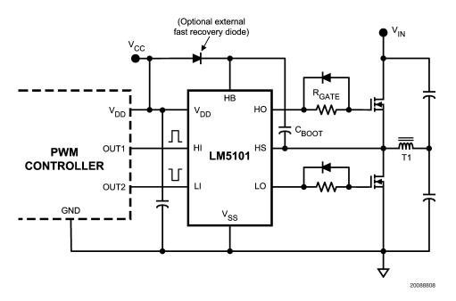
FIGURE 4. LM5101 Driving MOSFETs Connected in Half-Bridge Configuration
