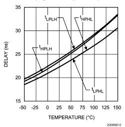
LM5101 Propagation Delay vs Temperature
