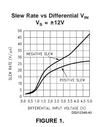
This effect is most noticeable at higher supply voltages and lower gains where incoming signals are likely to be large. This speed-up action adds stability to the system when driving large capacitive loads.
