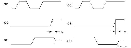
FIGURE 3. TRI-STATE Data Output Timing Diagram
