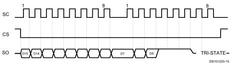
b) Reading Continuous Conversion - Two Eight-Bit Frames
