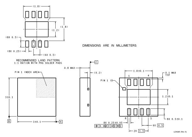
8-Lead Molded Lead Less Package
