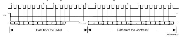
c) Writing Shutdown Control FIGURE 7. Timing Diagrams
