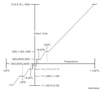
FIGURE 5. Temperature-to-Digital Transfer Function (Non-linear scale for clarity)
