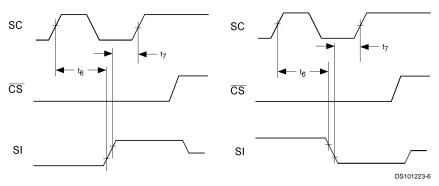
FIGURE 4. Data Input Timing Diagram
