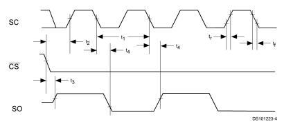
FIGURE 2. Data Output Timing Diagram
