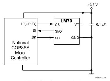
FIGURE 1. COP Microcontroller Interface
