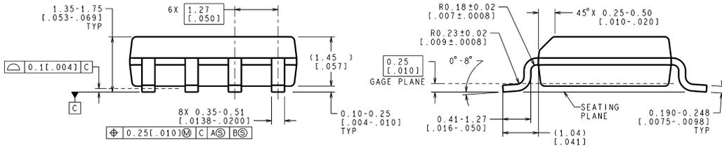
CONTROLLING DIMENSION IS MILLIMETER
