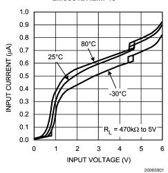
Reset Output Sink Current vs. Input Voltage LM8364BALMF45
