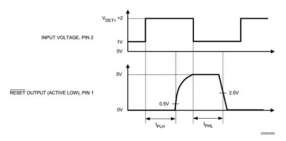
FIGURE 1. Propagation Delay Timing Diagrams
