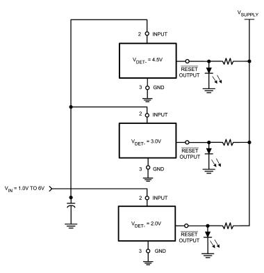
EACH LED WILL SEQUENTIALLY TURN ON WHEN THE RESPECTIVE VOLTAGE DETECTOR THRESHOLD (V $_{\rm DET.}$  +V $_{\rm HYS}$ ) IS EXCEEDED.
