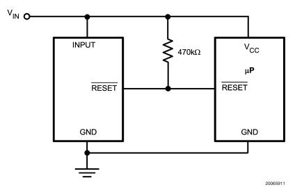
**Microprocessor Reset Circuit**
