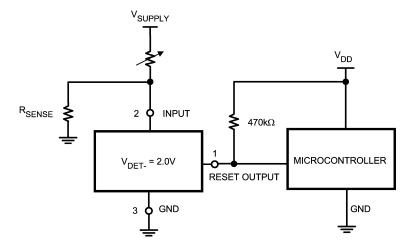
THIS CIRCUIT MONITORS THE CURRENT AT THE LOAD. AS CURRENT FLOW THROUGH THE LOAD, A VOLTAGE DROP WITH RESPECT TO GROUND APPEARS ACROSS  $R_{\rm SENSE}$  WHERE  $V_{\rm SENSE}$  =  $I_{\rm LOAD}$  \*  $R_{\rm SENSE}$ . THE FOLLOWING CONDITIONS APPLY:
