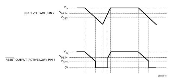
FIGURE 2. Timing Waveforms
