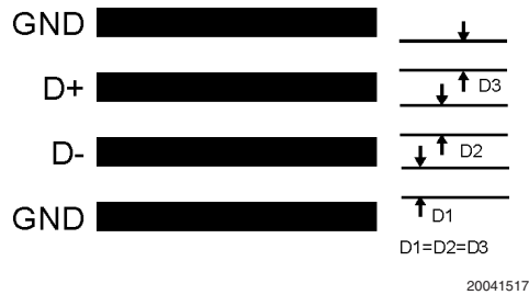
FIGURE 11. Ideal Diode Trace Layout
