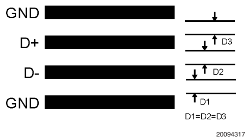
FIGURE 4. Ideal Diode Trace Layout
