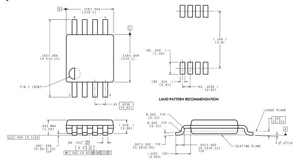
8-Lead Molded Mini-Small-Outline Package (MSOP), JEDEC Registration Number MO-187 Order Number LM95231CIMM or LM95231CIMMX NS Package Number MUA08A
