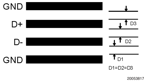
FIGURE 11. Ideal Diode Trace Layout
