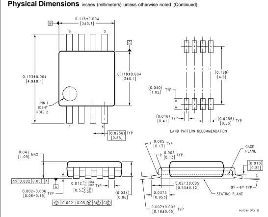
8-Lead (0.118" Wide) Molded Mini Small Outline Package Order Number LMC6442AIMM or LMC6442IMM or LMC6442IMMX NS Package Number MUA08A
