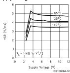
Negative Slew Rate vs Supply Voltage
