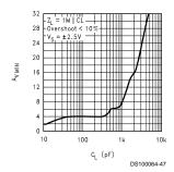
FIGURE 4. Minimum Operating Gain vs Capactive Load
