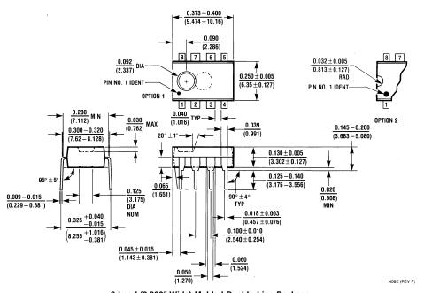
8-Lead (0.300" Wide) Molded Dual-In-Line Package Order Number LMC6442AIN or LMC6442INX or LMC6442INX NS Package Number N08E
