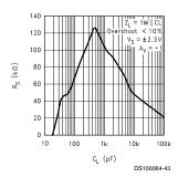
FIGURE 5. Isolating Resistor Value vs Capactive Load
