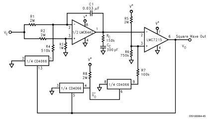
V <sup>+</sup> = 5V:  $I_{S}$  < 10 $\mu$ A, f/V $_{C}$  = 4.3 (Hz/V)
