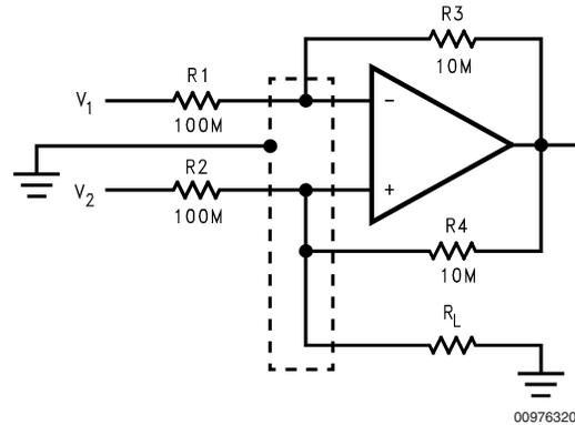
**FIGURE 9. Guard Ring Connections: Howland Current Pump**
