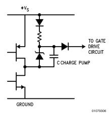
FIGURE 5. Internal Charge Pump Circuitry
