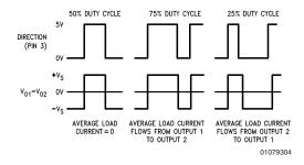
FIGURE 2. Locked Anti-Phase PWM Control
