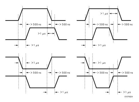
FIGURE 4. Transitions in Brake, Direction, or PWM Must be Separated by At Least 1 µsec
