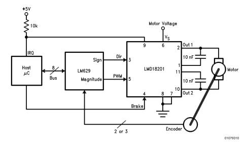
FIGURE 7. Basic Motor Driver
