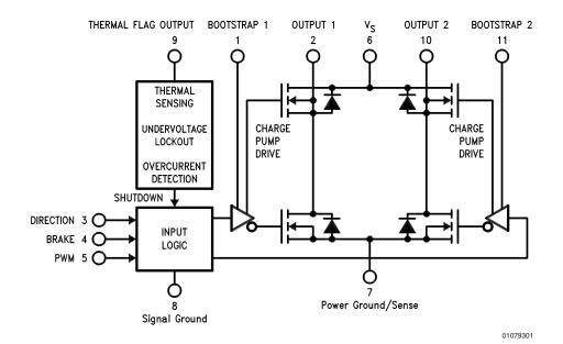
FIGURE 1. Functional Block Diagram of LMD18201
