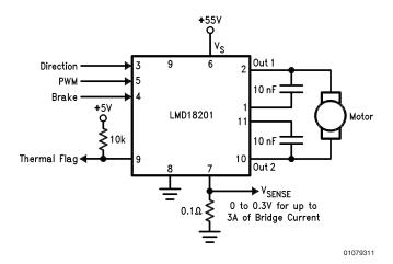
FIGURE 8. Current Sensing
