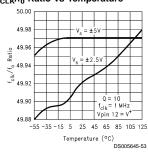
f<sub>CLK</sub>/f<sub>0</sub> Ratio vs Temperature
