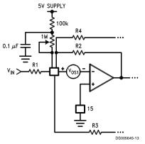
FIGURE 24. Method for Trimming  $V_{os}$
