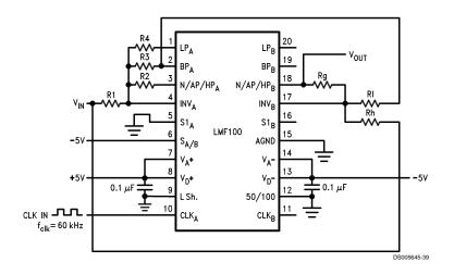
$\begin{array}{ll} R1 &= 100 \; k\Omega \\ R2 &= 1 \; k\Omega \\ R3 &= 100 \; k\Omega \\ R4 &= 100 \; k\Omega \\ Rg &= 10 \; k\Omega \\ RI &= 10 \; k\Omega \end{array}$
