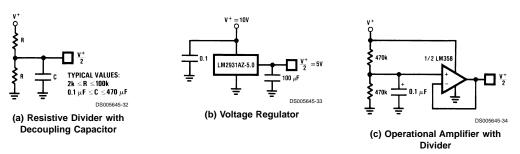
FIGURE 21. Three Ways of Generating V+/2 for Single-Supply Operation
