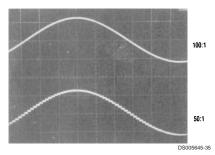
FIGURE 25. The Sampled-Data Output Waveform
