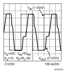
FIGURE 2. Overload Recovery Waveform
