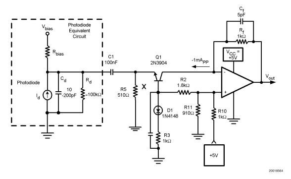
FIGURE 3. Single Supply Photodiode I-V Converter
