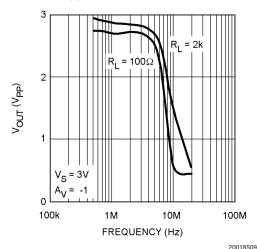
Closed Loop Small Signal Frequency Response for Various Supplies
