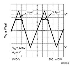
FIGURE 1. Input and Output Shown with CMVR
