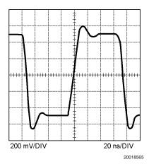
FIGURE 4. Converter Step Response (1V<sub>PP</sub>, 20 ns/DIV)
