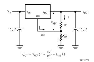
FIGURE 1. Basic Adjustable Regulator
