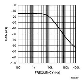
FIGURE 10. Lowpass Filter Frequency Response
