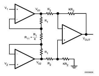
FIGURE 1. Instrumentation Amplifier
