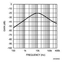
FIGURE 11. Bandpass Filter Frequency Response
