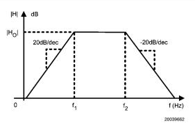
FIGURE 8. Bandpass filter Transfer Function
