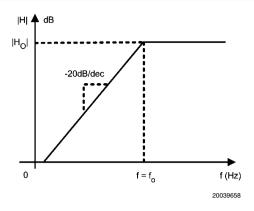
FIGURE 6. Highpass Filter Transfer Function
