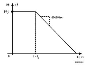
FIGURE 4. Lowpass Filter Transfer Function
