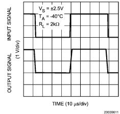
Non-Inverting Small Signal Pulse Response
