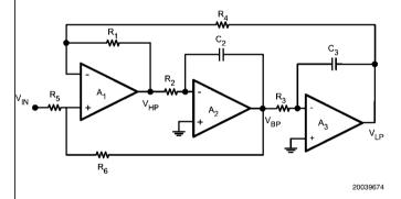
FIGURE 9. State Variable Active Filter
