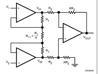
$V_0 = -K (2a + 1) (V_1 - V_2)$
