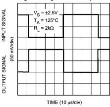
**Inverting Large Signal Pulse Response**
