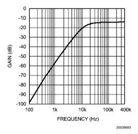
FIGURE 12. Highpass Filter Frequency Response
